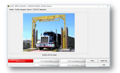
The Camera tab displays the image taken during the occupancy or a representation of the type of vehicle. If a camera is enabled, then the image captured during the occupancy will be displayed. The image may not be displayed immediately depending on the camera's trigger time. If the camera is disabled, then either a picture of a truck or train car will be
