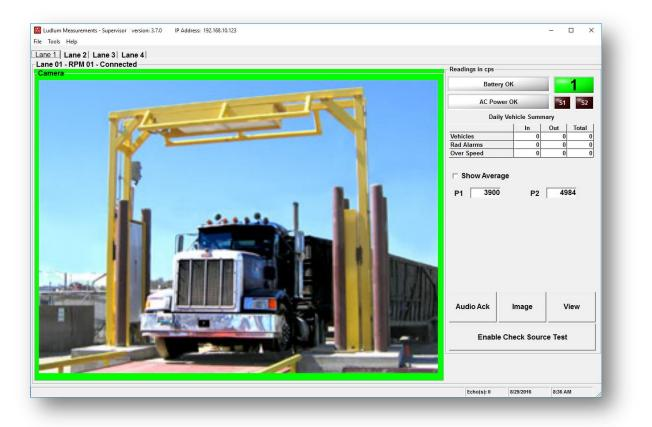
lane. Each tab displays a camera image, battery and AC power status, infrared sensor indicators, and vehicle counts including number of radiation alarms and over-speed alarms, and the current background readings for each panel. There
