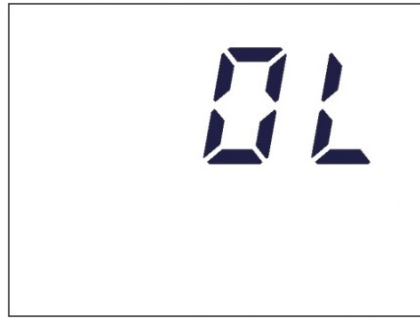
Figure 2.7: Detector Overload Alarm (Display Will Flash)
