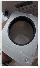
If the detector mounting and O-ring has contamination, an alternative and more extensive process of removing the entire cylindrical detector assembly and shield from the Model 3030P chassis can also be accomplished. Following the same steps above, power down and remove the cover of the Model 3030P and remove the connectors and the lead shield bracket.
